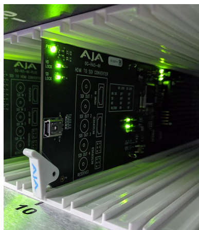
Figure 9. Fully Inserted Card with Locked Plastic Tab
