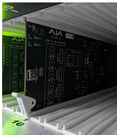
Figure 9. Fully Inserted Card with Locked Plastic Tab
