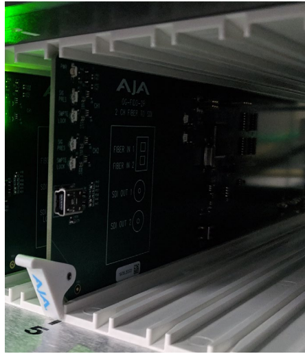
Figure 7. Fully Inserted Card with Locked Plastic Tab
