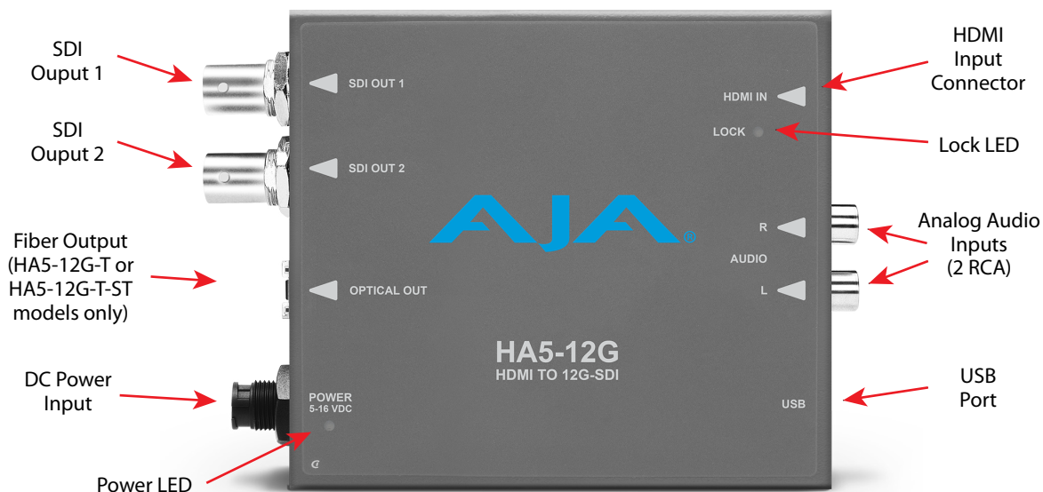
Figure 2. HA5-12G Converter Connections
