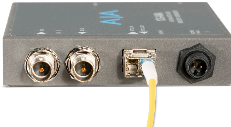
Figure 2. 12G-AM to Fiber LC Single Channel SFP Example
