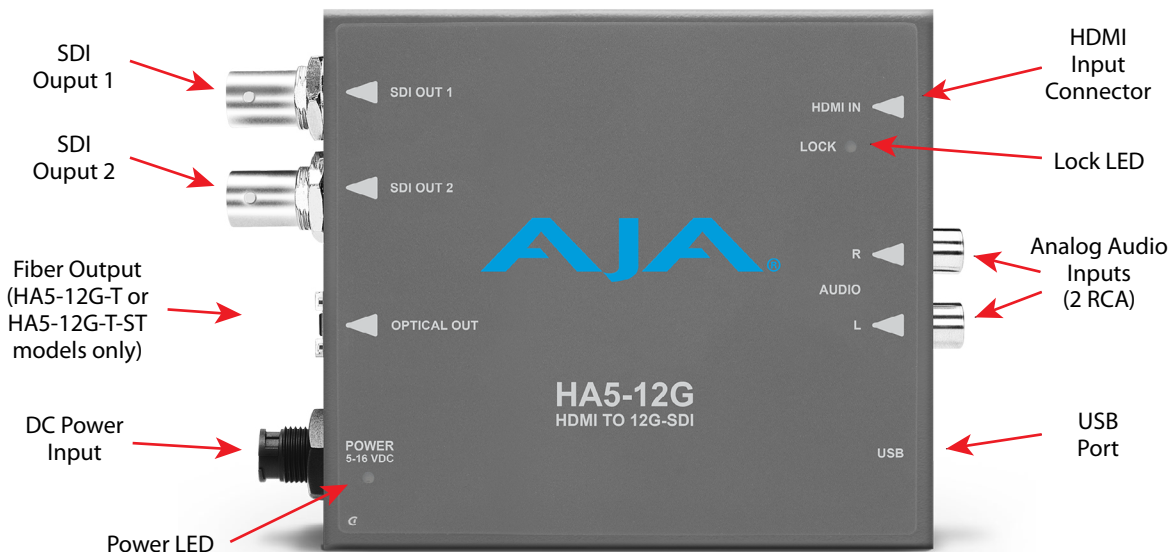
Figure 2. HA5-12G Converter Connections
