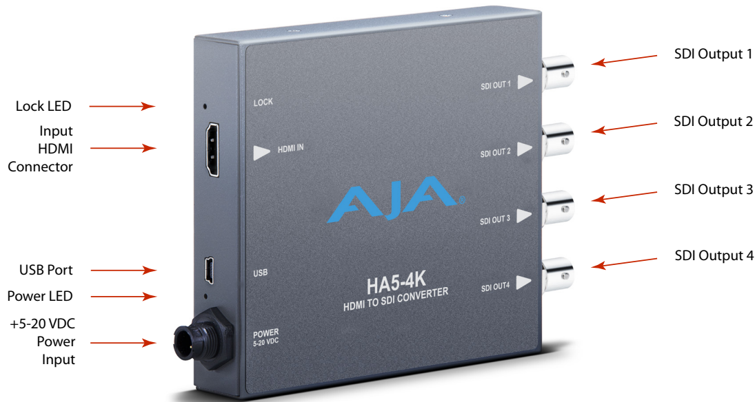
Figure 2. HA5-4K Converter Connections
