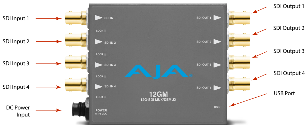
Figure 2. 12GM Converter Connections
