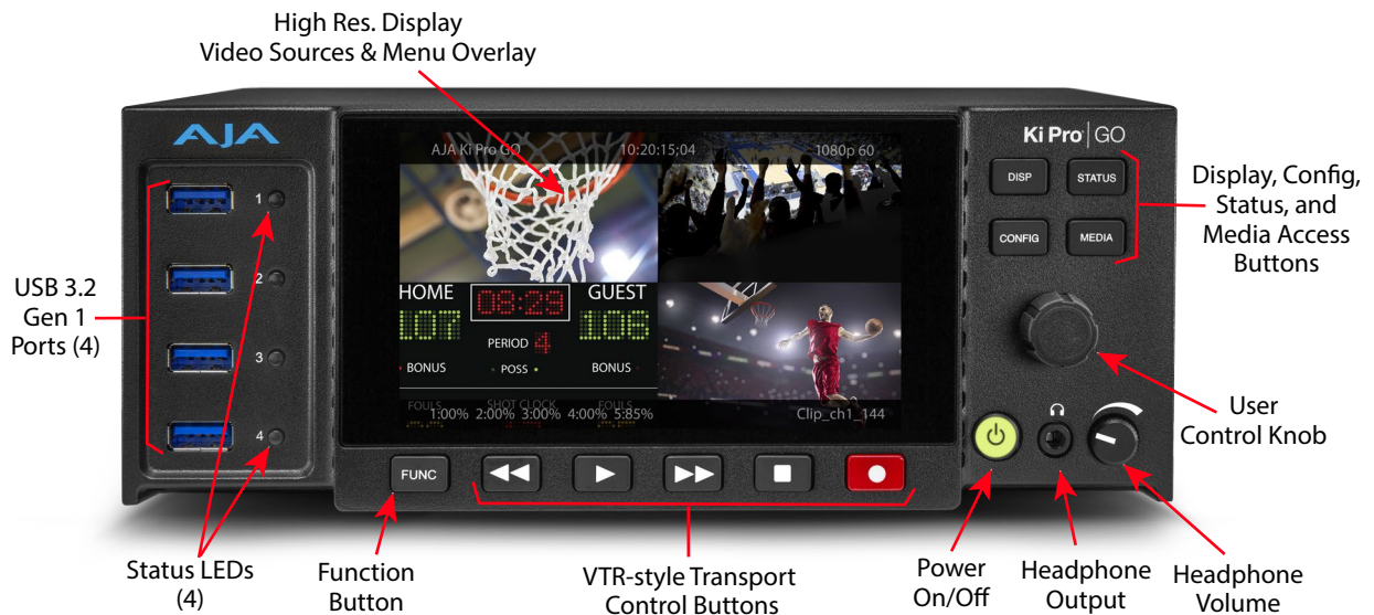
Figure 1. Ki Pro GO Front Panel
