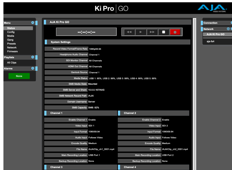
Figure 19. Status Screen, with SMB Mounted
