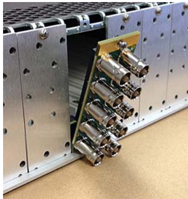
Figure 4. Rear Card Inserted Into Frame Seating Slot
