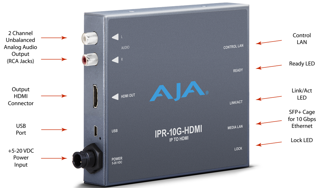
Figure 2. IPR-10G-HDMI Connections
