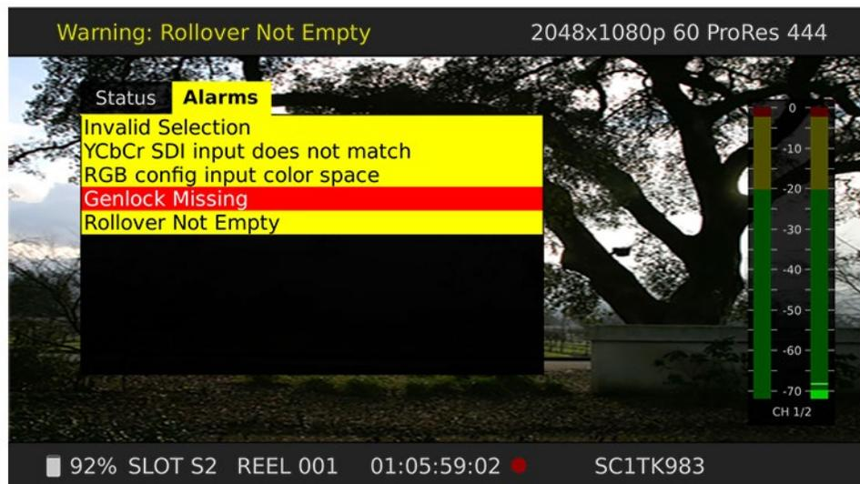
Once there is a Ki Pro Ultra Plus alarm active, the STATUS button light will blink for as long as the alarm is present. This alerts you so you'll know the reasons for the alarm condition are still active—you can then check the ALARMS display by pressing the STATUS button and using the User Control Knob to scroll to the ALARMS tab.
