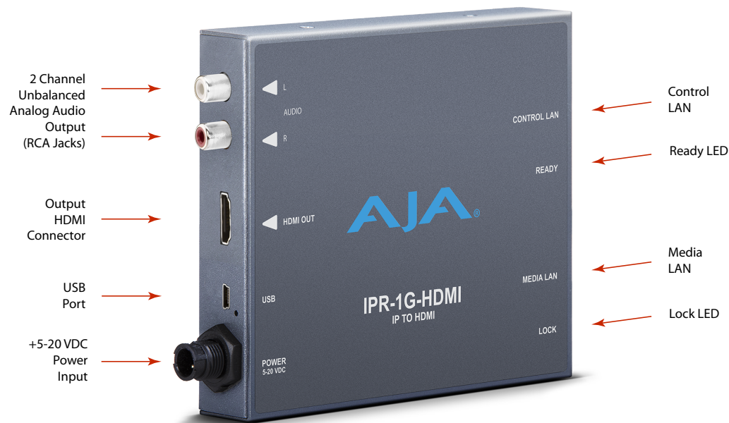
Figure 2. IPR-1G-HDMI Connections
