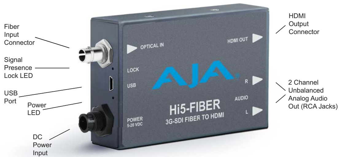
Figure 2. Hi5-Fiber Converter Connections
