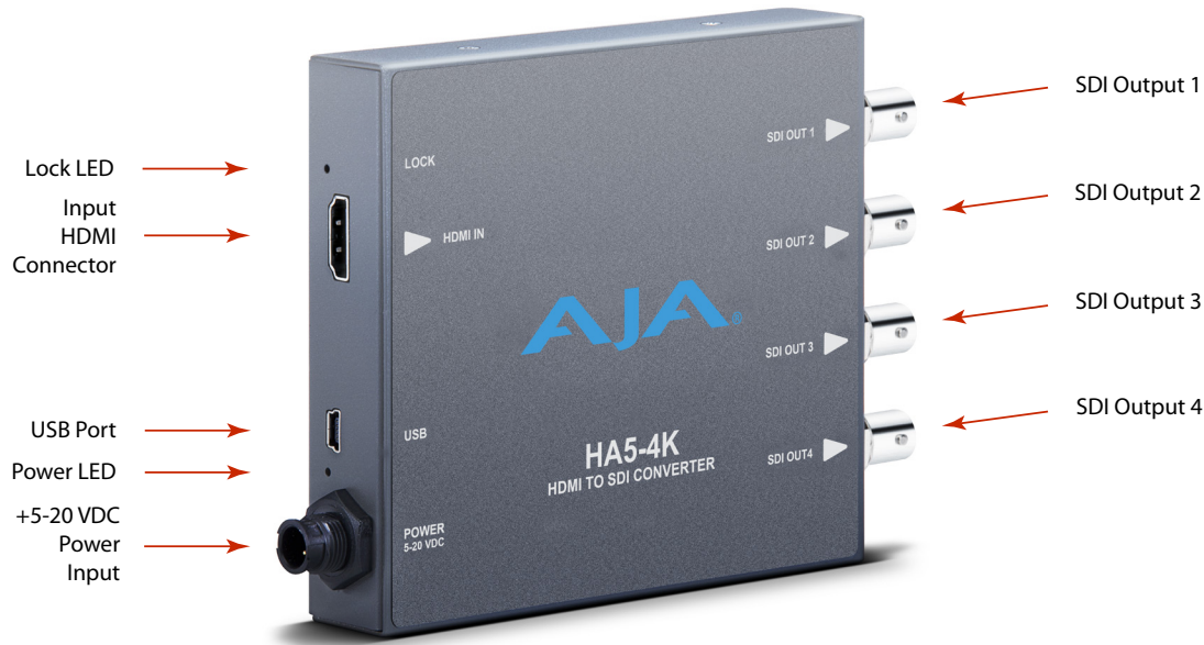
Figure 2. HA5-4K Converter Connections
