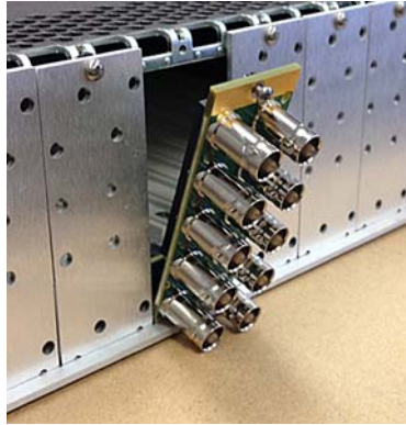
Figure 2. Rear Card Inserted Into Frame Seating Slot
