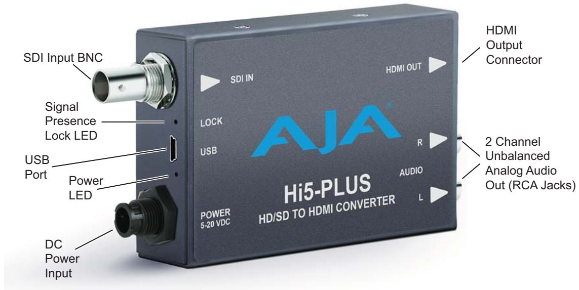
Figure 2. Hi5-Plus Converter Connections
