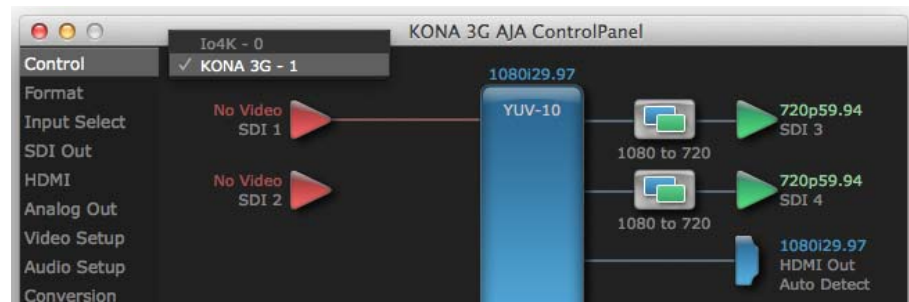
Figure 57. Control Panel Screen Showing Multiple AJA Devices
