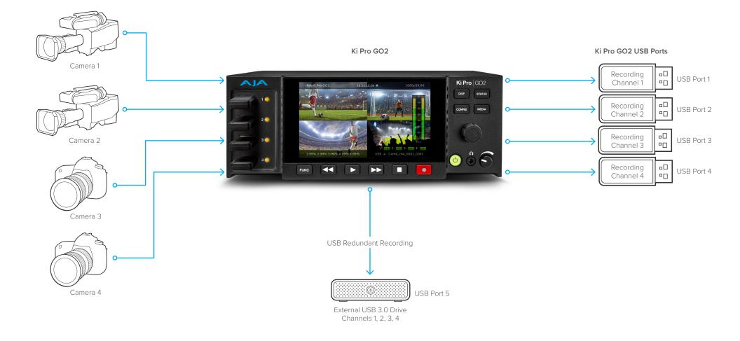
USB Recording Mapping: Four Camera Feeds, Primary and Backup Recordings
